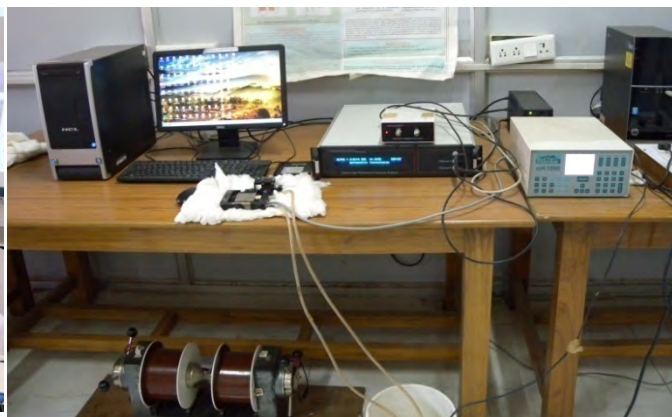
Wide frequency and impedance range high performance Impedance Analyzer- Novocontrol (Alpha-A)
